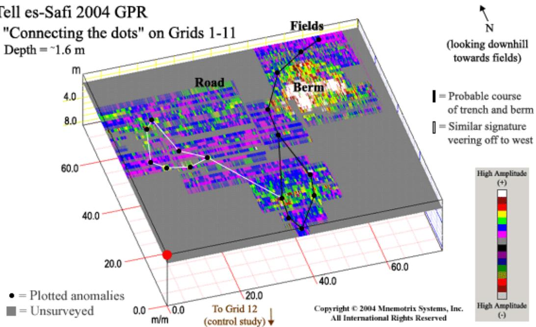
**Figure 4: After studying the individual grids, we were able to plot the signatures labeled in each to trace the probable course of the trench and berm. A similar signature seemed to veer off to the west in Grids 2, 3, and 4. Ground truth excavation will be the key to understanding the true nature of these GPR anomalies.**
